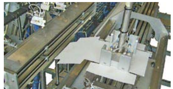
Tray erecting station
