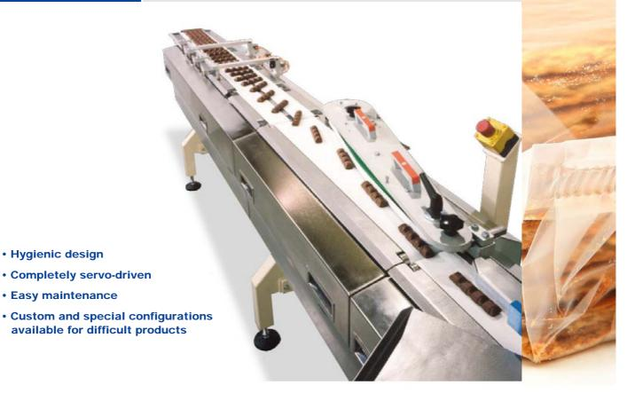
Belt groups controlled by an independent Servo Motor in full coordination with the flow-wrapper
