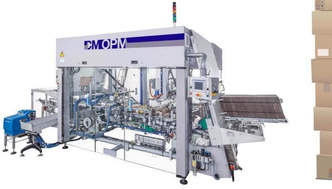
The WA series consists of wrap-around automatic machines for products, packaged by wrapping machines or side loading machines, in fluted corrugated paperboard and /or trays.
